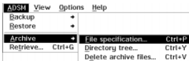
Figure 23. Selecting Archive by File Specification from the ADSM Menu
