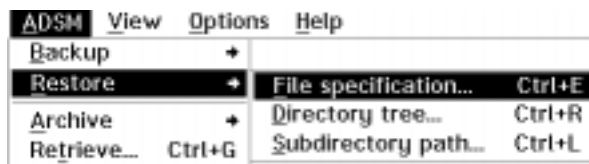
Figure 16. Selecting Restore by File Specification from the ADSM Menu
