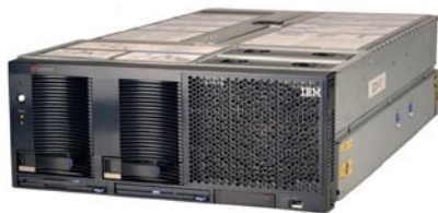
Virtual servers on rack-dense IBM xSeries systems can take the place of a room full of physical machines.
