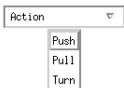
Figure 7-3 Example of menu button widget (DtMenuButton)
