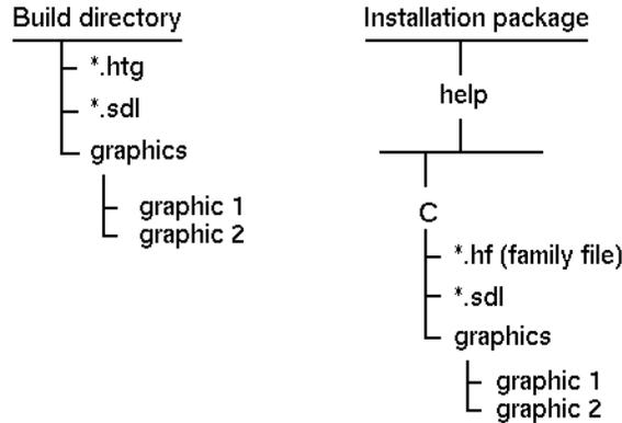
Figure 13-2 Relationship of build directories and installation package
