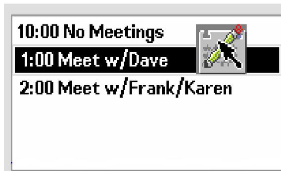
Figure 3-7 Example of a scrolling list with an item selected for dragging
