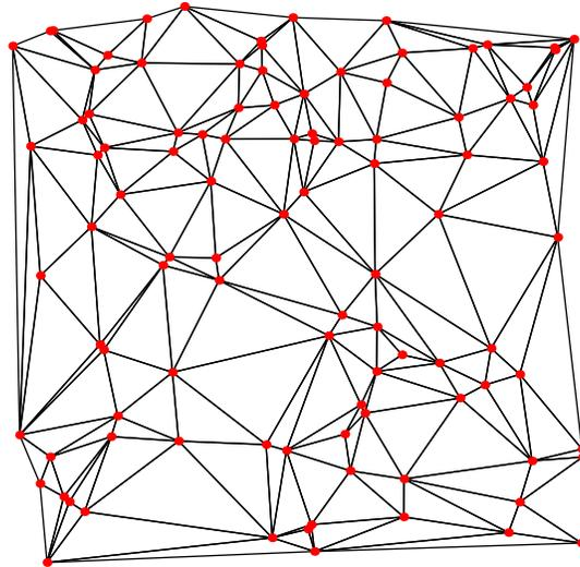
The example `Gouraudcontour` illustrates how to produce color density images over such irregular triangular meshes. `Asymptote` uses a robust version of Paul Bourke's Delaunay triangulation algorithm based on the public-domain exact arithmetic predicates written by Jonathan Shewchuk.
