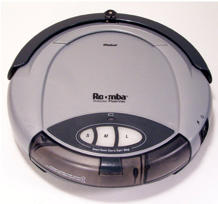
Figure 3.2: Roomba of first generation: a vacuum cleaner
