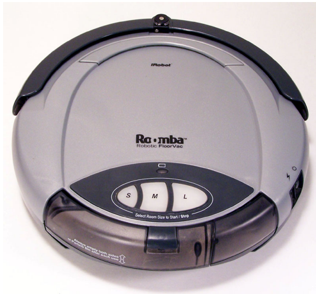
Figure 3.2: Roomba of first generation: a vacuum cleaner
