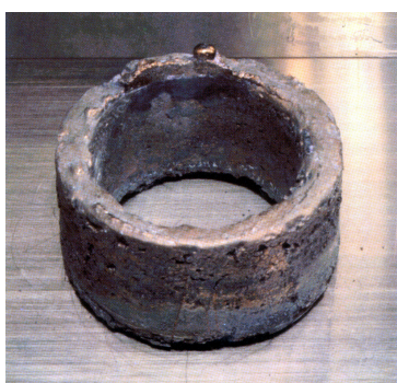
A ring of weapons-grade 99.96% pure electrorefined plutonium, enough for one bomb core. The ring weighs 5.3 kg, is ca. 11 cm in diameter and its shape helps with criticality safety.
