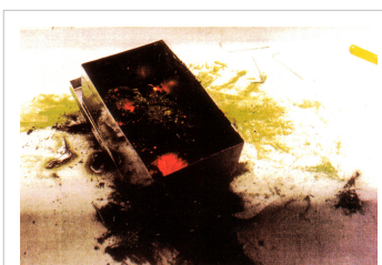
Plutonium pyrophoricity can cause it to look like a glowing ember under certain conditions.
