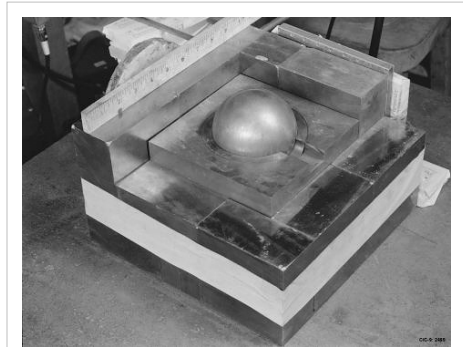
A sphere of simulated plutonium surrounded by neutron-reflecting tungsten carbide blocks in a re-enactment of Harry Daghlian's 1945 experiment
