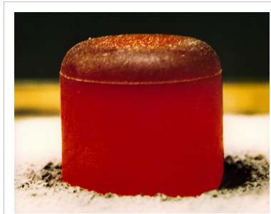
Image of (mostly) thermally isolated, RTG pellet glowing red hot because of incandescence.
