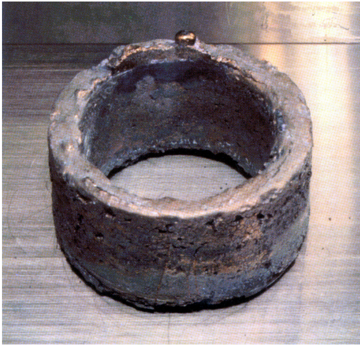
A ring of weapons-grade electrorefined plutonium, with 99.96% purity. This 5.3 kg ring is enough plutonium for use in an efficient nuclear weapon. The ring shape is needed to depart from a spherical shape and avoid criticality.
