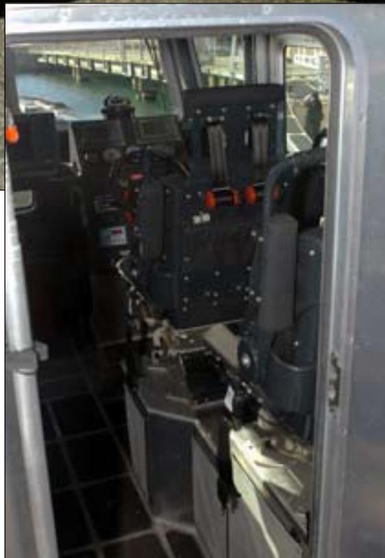
When out on patrol, the crew can sit in shock mitigating seats that relieve stress on the kness as well as stay cool in the air conditioned cabin.
