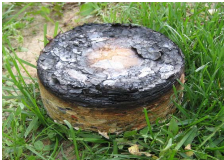
Fig. 15. Photograph of the biomass log after partial gasification.
