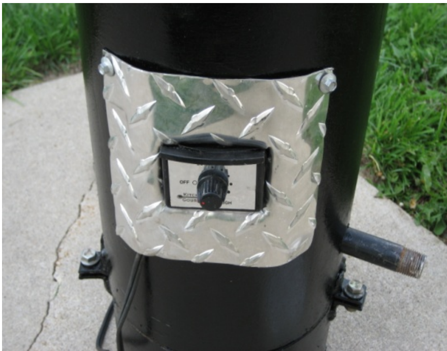
Fig. 12. Close up of the heating element temperature control.
