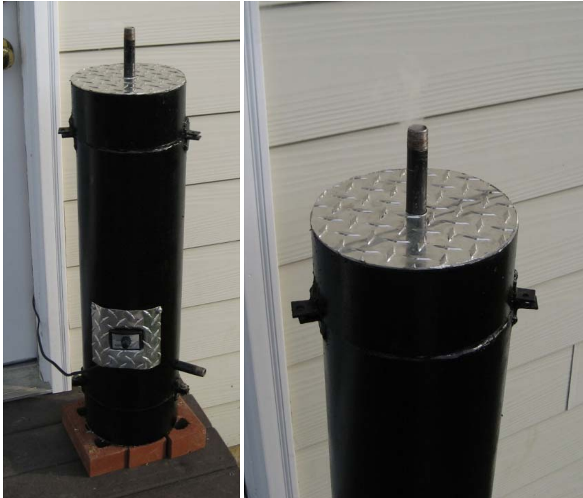
Fig. 14. Image of test setup (left), and photograph of syngas leaving outlet (right).
