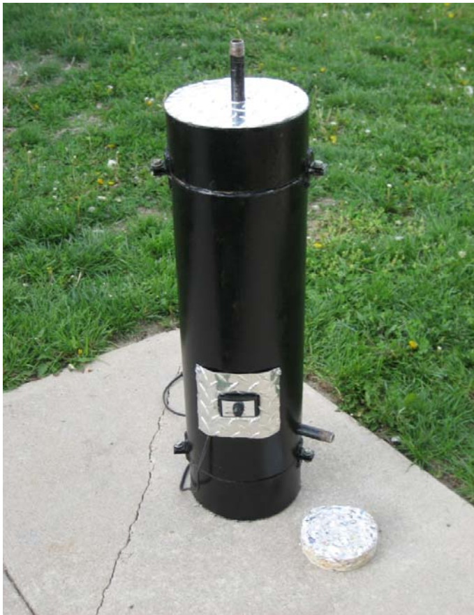
Fig. 10. Photograph of the entire gasifier prototype and compressed log.
