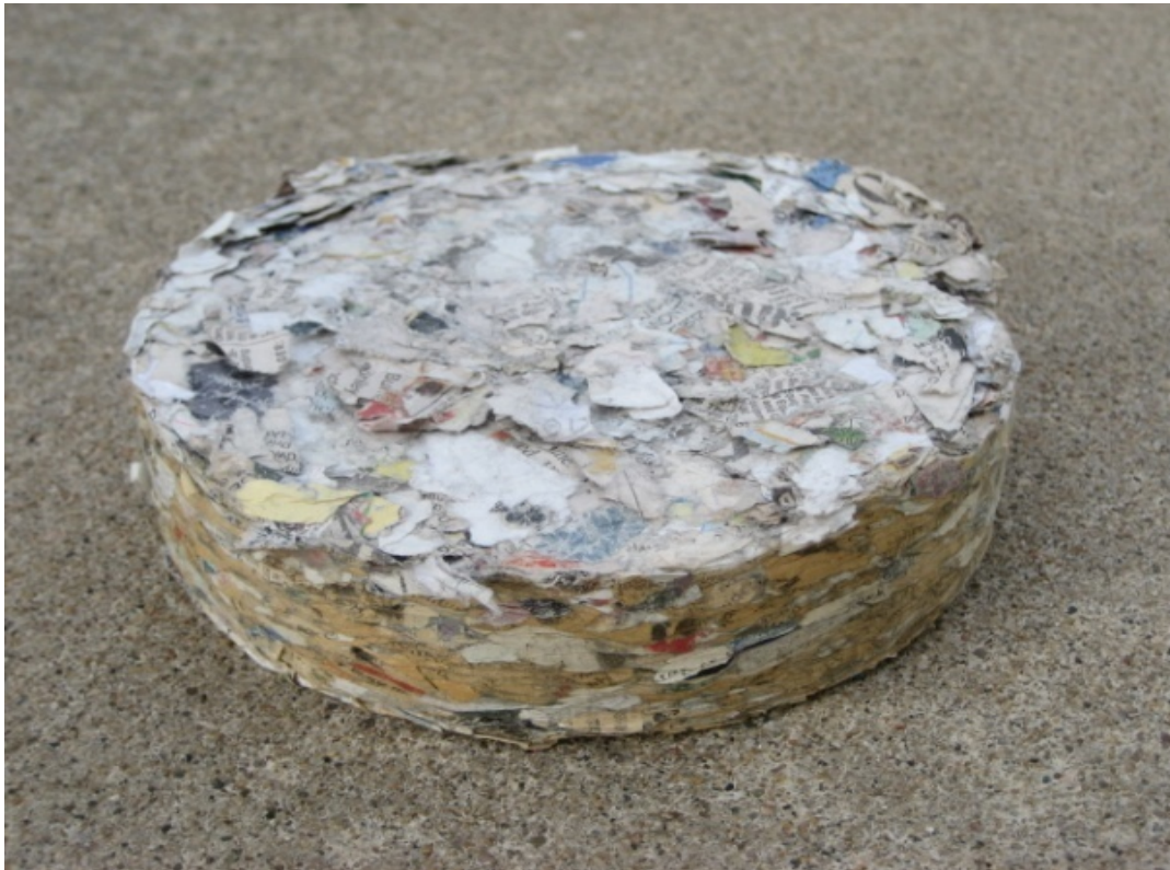
Fig. 13. Photograph of compressed biomass log used for testing.
