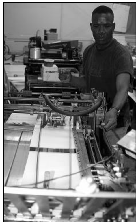
Errol Parkes puts the printed and cut spreads through DAPS' amazing folding machine.
