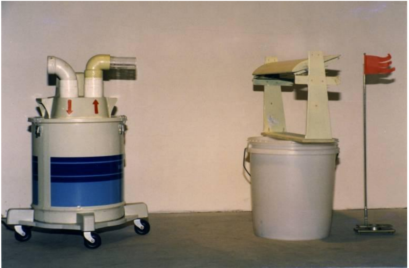
2 Above photos, demonstrate something different. Unlike an airplane wing that is fixed to the plane, an airfoil is suspended horizontally on four springs and is aligned with the air flow. When the air blower is switched on, the stream of air presses the front-edge down and raises the top-rear up. This emphasizes the explanation of Fig. D. on the previous page.
