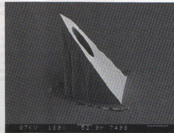
Figure 7.14 Microfabricated microneedle. (Photo courtesy of Micronit, Inc.)
