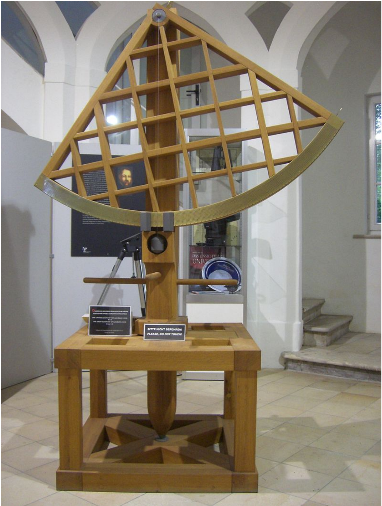
Smaller scale reconstruction of Tycho's Augsburg Quadrant in Römerturm in Göggingen - the celestial object is sighted along the upper right-hand straight edge and its elevation read off where the plumb-line crosses the curved vernier scale.
