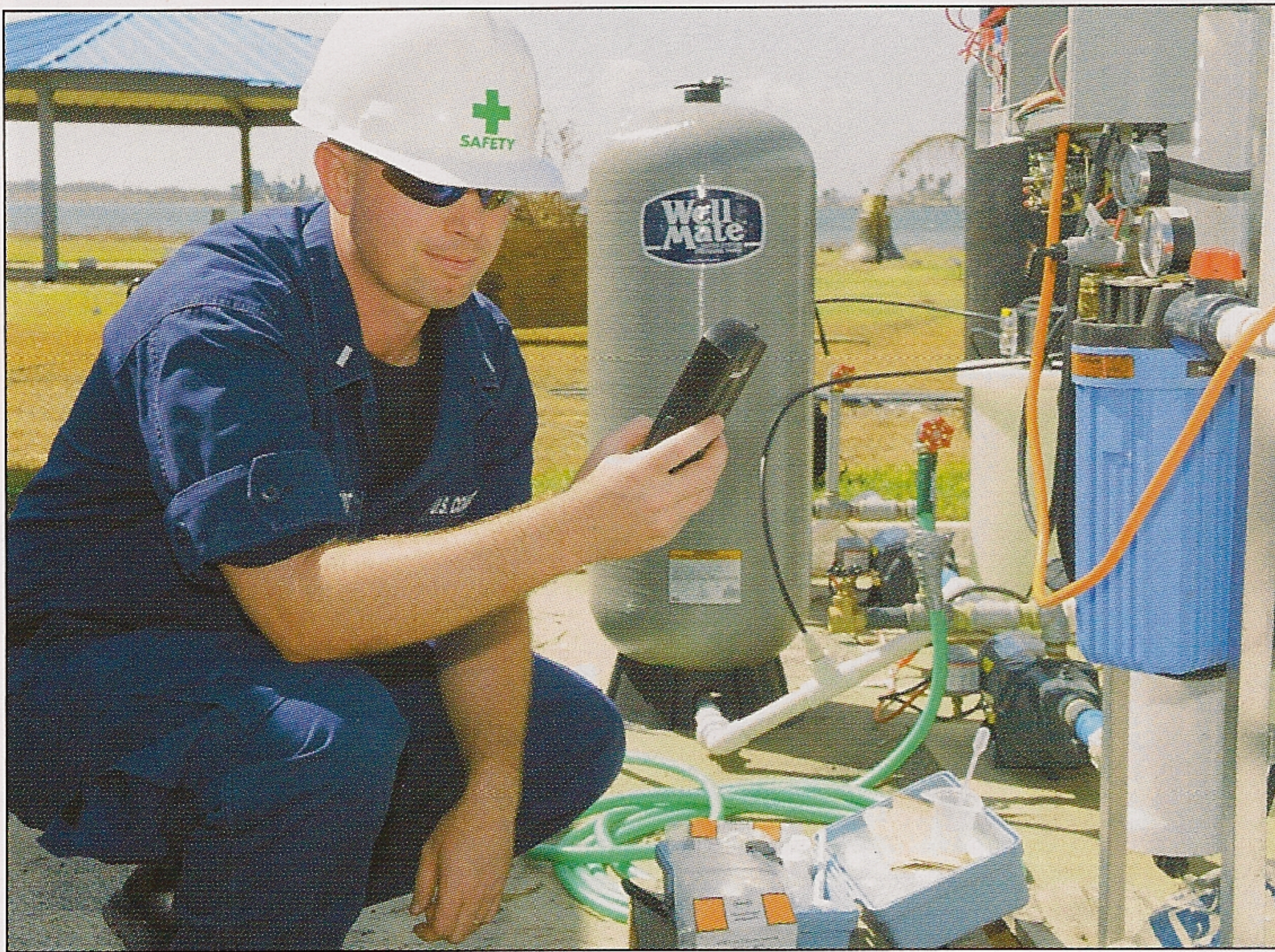
LTJG Jon Bernhardt, a reservist from MLC LANT, samples chlorine at Station Galveston as ad-hoc housing and water treatment was established by a team from MLC. The station's housing was wiped out by Hurricane Ike.
