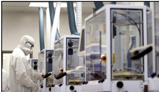
Wafer loading on the oligonucleotide synthesizer and removal on completion
