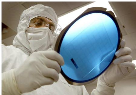
Inspection of the wafer prior to dicing and wafer mounting on the dicing saw
