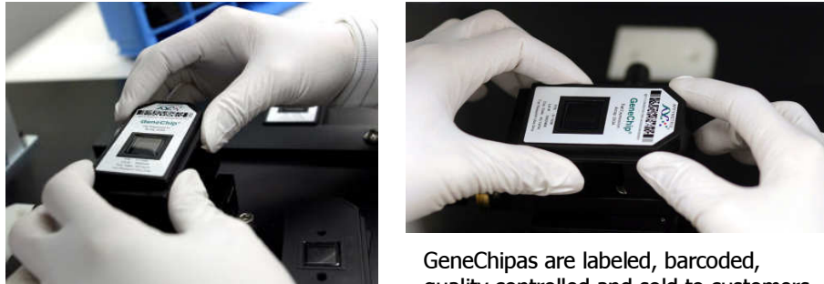
The wafer is diced and individual chips are mounted into plastic GeneChip cartridges
