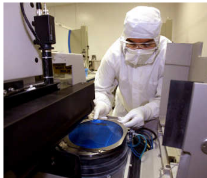
Wafer loading on the oligonucleotide synthesizer and removal on completion
