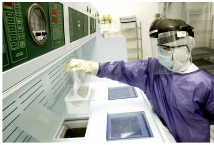
Transfer of wafers at the cleaning wetbench and application of antireflective coat
