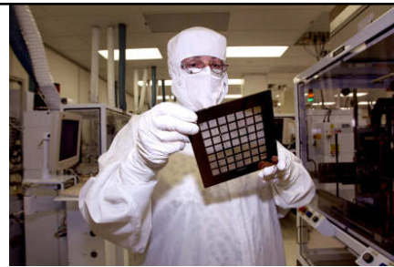
Wafer loading on the oligonucleotide synthesizer and removal on completion
