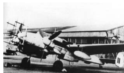
Top: German Junkers JU88G night bomber in flight; Left: Nose of the JU88G night bomber bristled with antennas; Right: German Messerschmitt Me110G4 night fighter with nose antennas.
