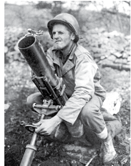
The 4.2-inch Chemical Mortar (Four-Deuce) fired high explosive and white phosphorus rounds. The 4.2-inch mortars of the 83rd Chemical Mortar Battalion provided fire support to the Rangers throughout the campaign in Italy.
