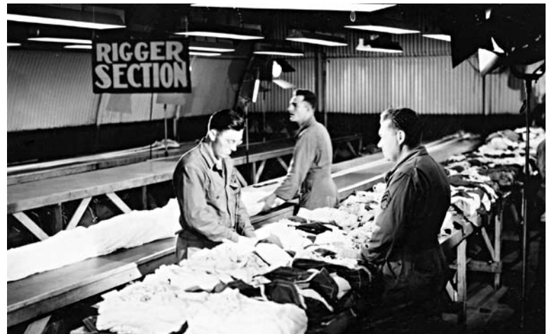
Men of the Rigger Section pack parachutes. Notice the bright lighting which helped to ensure that the parachutes were packed correctly.
