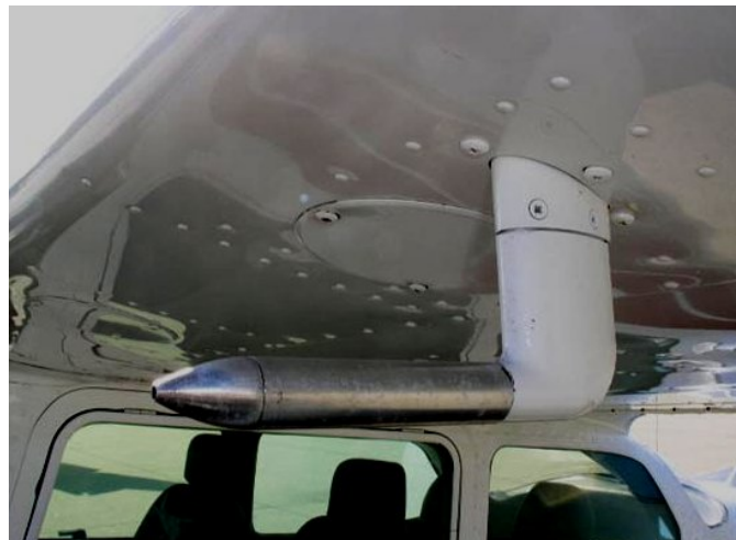
A Pitot tube underneath the wing of an aircraft.
