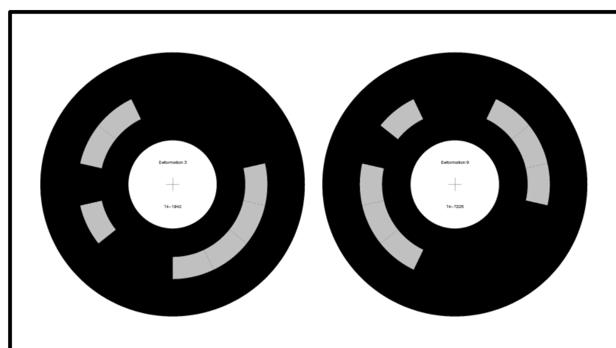
Two blobs with IDs. SwisTrack detects their position, orientation and ID.
