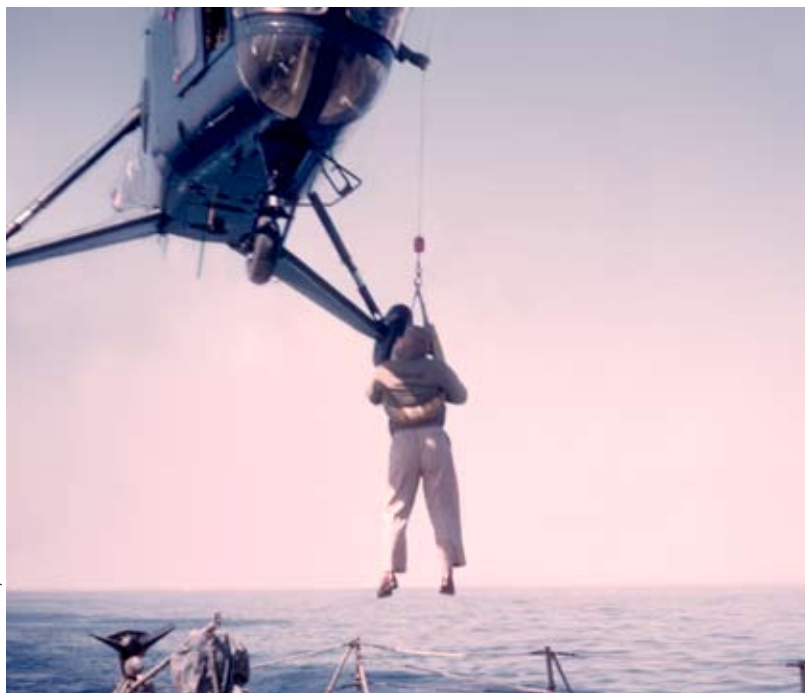
U.S. Navy RH-5 Sikorsky helicopter effecting pilot rescue with sling and "horse collar."
