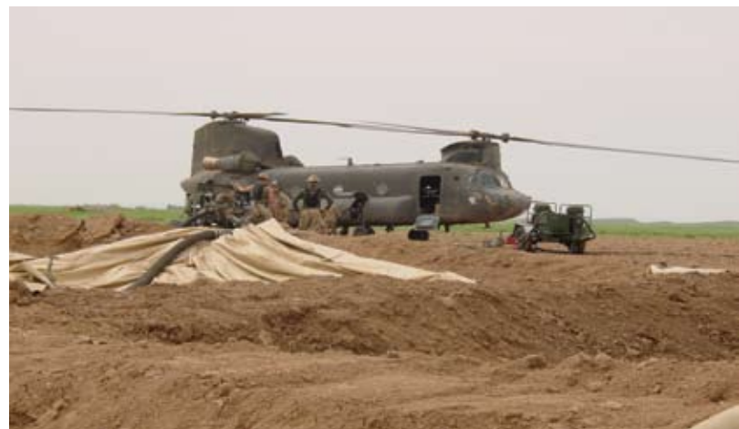
The TF Support operations refueled aircraft as required. Refueling a CH-47 helicopter of the 101st Airborne Division.
