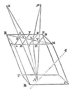
Hence, that I might examine the nature and difference of both. I put, upon some Object, as the point A, the Prisme of my Double refracting Chrystal N, P, R, Q, T, B, S; and the Eye M, being perpendicularly posited over the upper plain of the Prisme N, P, R, Q, I noted, whether there was any Refraction of the point A, (for the usual Lows of Retraction teach, that there is none.) But the Perpendicular
