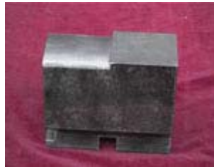
Combination Fullering to flat die
