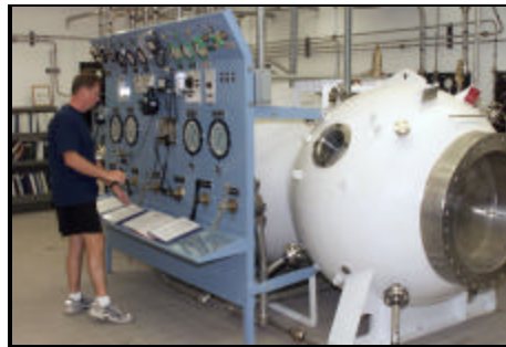
Chief Petty Officer Bob Lambertsen lowers the compression depth of the new recompression chamber from 10 feet to zero in order to open it.
