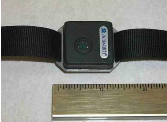
Figure 3-4. Image of an Actiwatch activity monitor that is shown next to a ruler to demonstrate the size of the Actiwatch.
