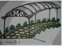
PRECAST CONCRETE PAVERS BLOCK LAID ON COMPACTED LAND
