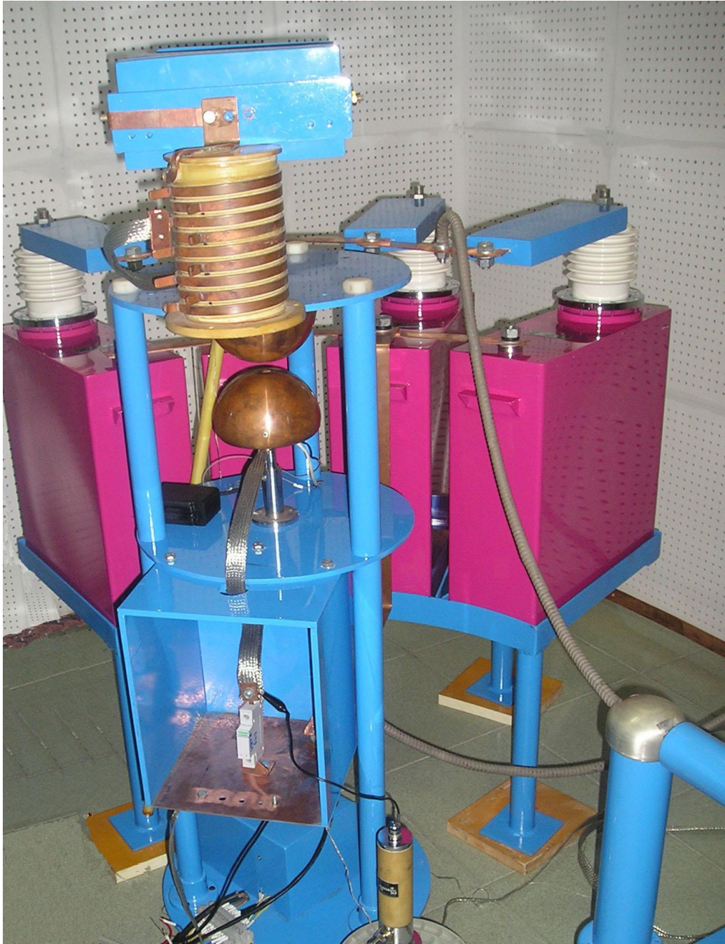
This is the 60 KA Surge Generator test lab for SPD application test.
