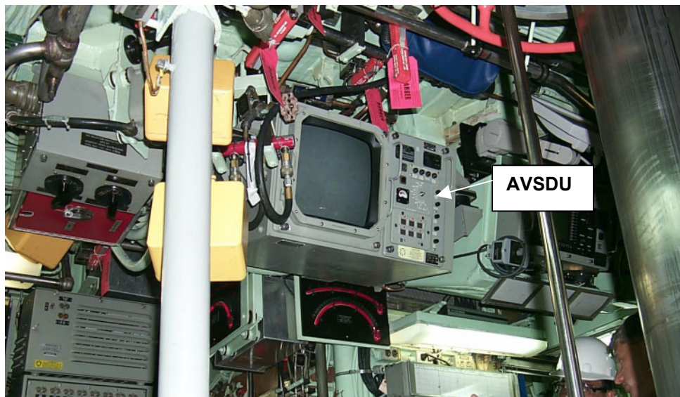
Figure 4. The Analog-Video Signal Display Unit, or AVSDU, was a sonar repeater installed near the Greeneville 's periscope platform. On the day of the accident, the AVSDU was not working. (U.S. Navy photo)
