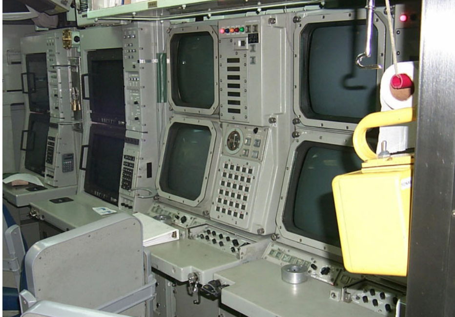
Figure 5. Each sonar workstation, or stack, had two monitors. The two stacks at right displayed system input from hull-mounted arrays. (U.S. Navy photo)
