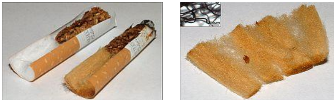
Fig. Cigarette Filters n Cellulose acetate fiber bundle.
