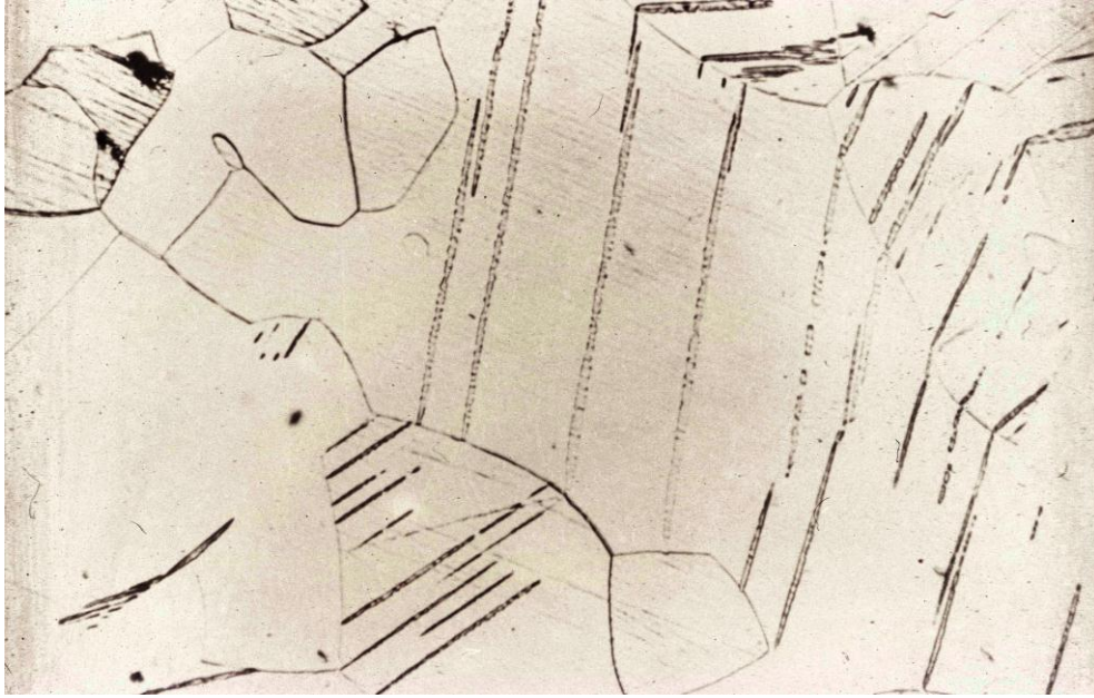
Fig 58. Neumann bands in rolled 3% Si steels ( after P.Moore 16 )
