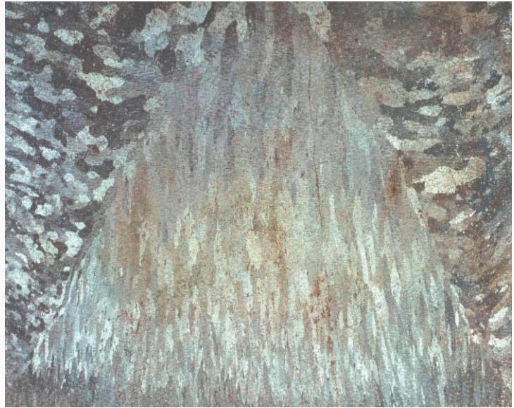
Fig 6. Section of a con.cast slab
