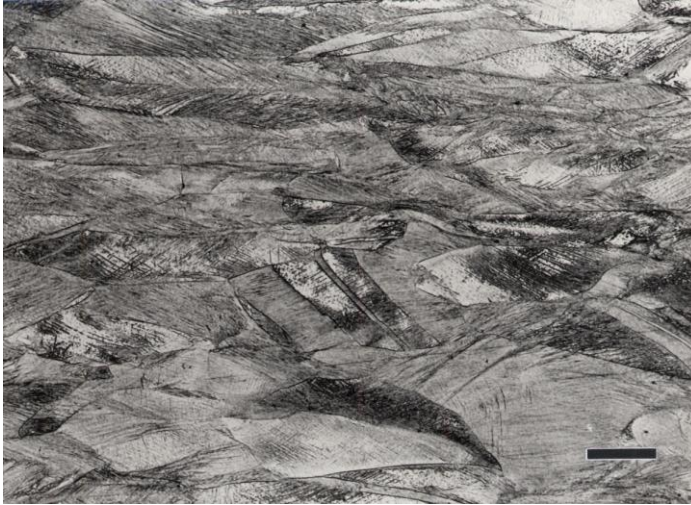
Fig 72 c cold rolled by 50%
