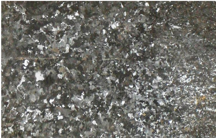
showing fine equi-axed ferrite grains
