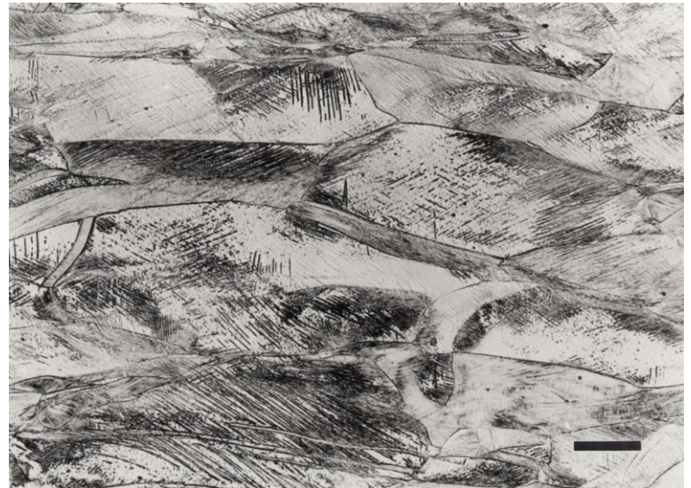
Fig 72b cold rolled by 40%
