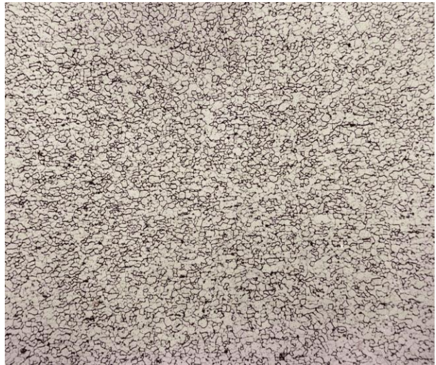
Fig 26. Sample in Fig 25 held for a longer time at a higher temperature to ensure complete recrystallisation
