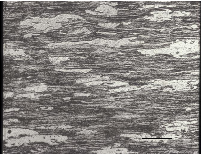
Fig 30. Elongated recrystallised ferrite grains within the cold rolled structure (scale=100 \mu m)
