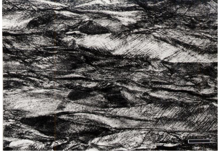
Fig 72 d cold rolled by 60%
