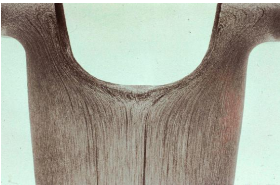
Fig 40 Fibrous grain flow
