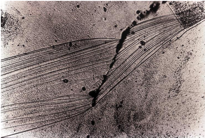
Fig 53 ----- 50\mu\text{m} The course of boundary migration seen here is evidently influenced by a line of obstacles such as dislocations, as revealed by the etch pits. Another interesting point to note in Fig52 is that the spacing between successive positions of the boundary increases with the ageing time ( compare Figs 52 a to c).
