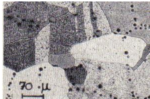
Figs 45 & 46. Fe- ~2at % In alloys showing \alpha veining(same mag)
