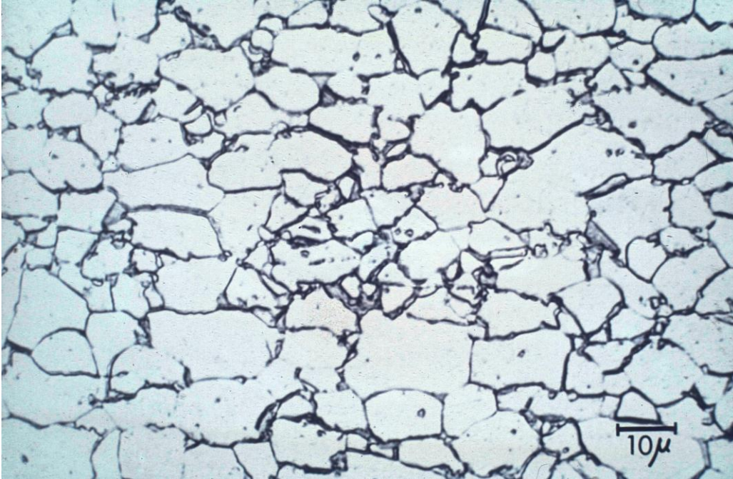
Fig 15. Dual phase steel. The light areas are ferrite and the dark areas are bainite or martensite.
