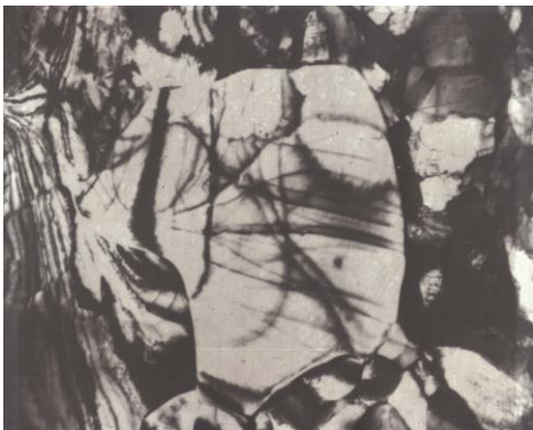
Fig 22. Microstructure of a low carbon steel slowly heated to 500^{\circ}\text{C} ( after Adrian Dunn/ Univ.Liverpool 11 )
