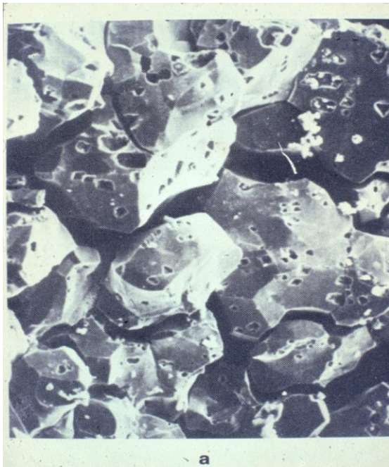
Fig 85 Failure at the grainboundaries & severe pitting on the grain surfaces.
