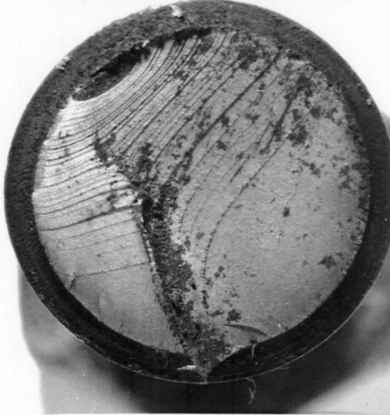
striation spacing increases with the stress range
